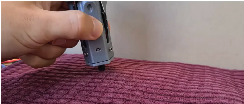
Image 1. FeelScan that registers texture on different surfaces.
